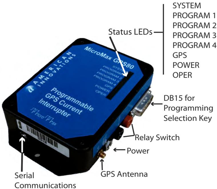
**Figure 1. GPS80 Interrupter**
