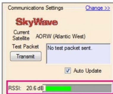
Figure 6-1. Satellite Signal Strength
