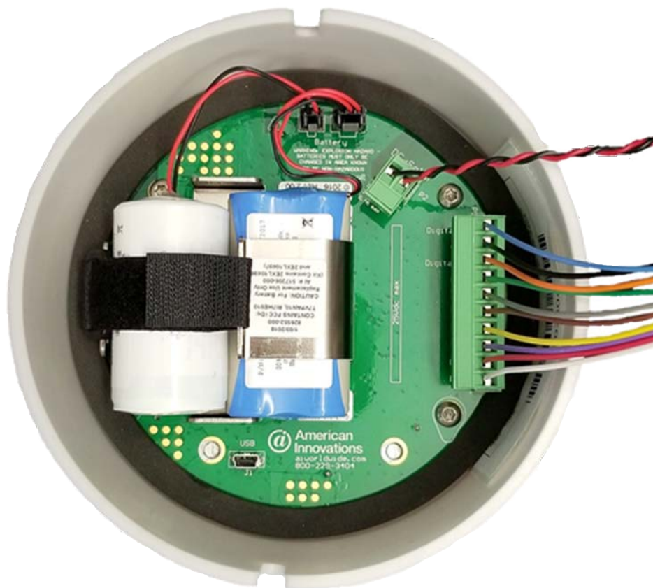
Figure 4-3. Battery Bracket and Battery Placement (wired with optional Solar connection)
