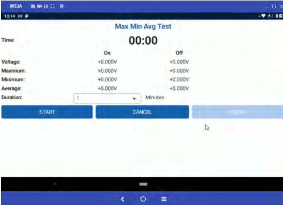
Figure 1-2. Max Min Avg Test Window
