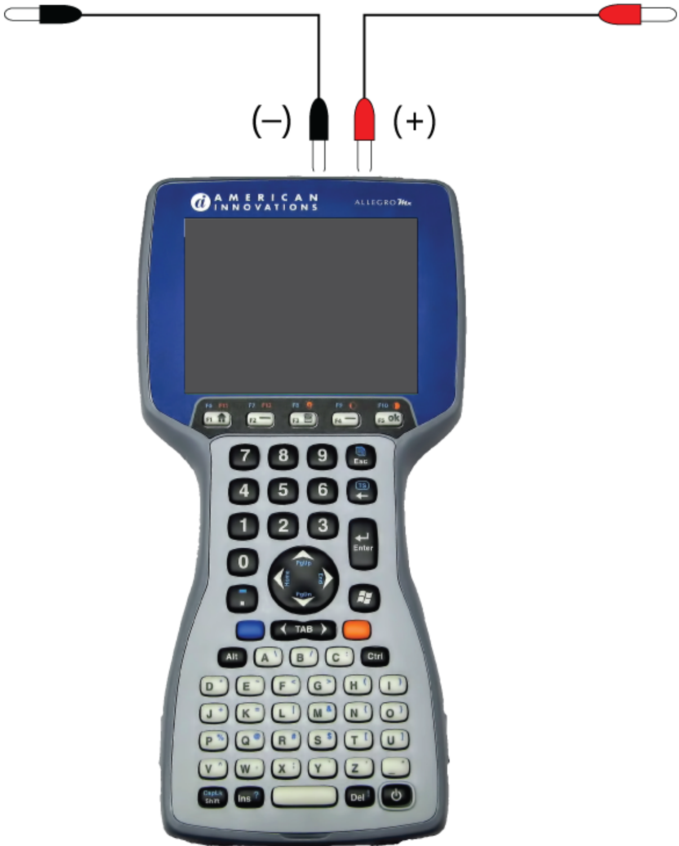
Figure 2-1. Allegro MX Connections Configuration for DVM
