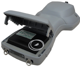
Figure 1-2. Install Battery Pack
