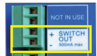
Remote Monitoring Unit Relay Input
