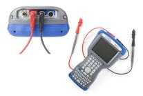
Figure 2-1. Allegro QX Connections Configuration for DVM
